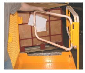
Lift the gate to allow the slots to slide onto the pegs welded to the toeguard.
