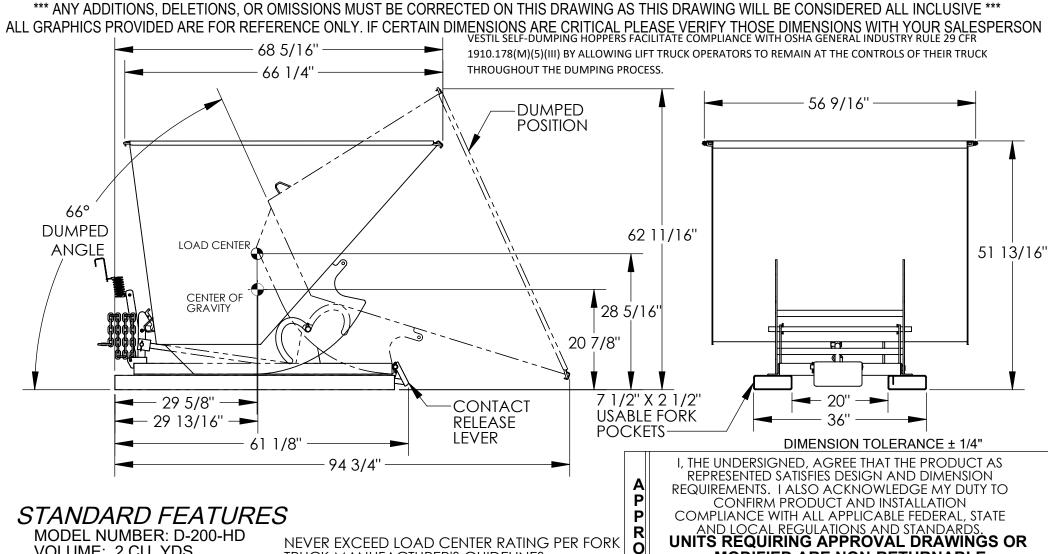
VOLUME: 2 CU. YDS. CAPACITY: 6,000 LBS. OVERALL WIDTH: 56 9/16" OVERALL LENGTH: 68 5/16" OVERALL HEIGHT: 51 13/16" PULL CABLE IS AT LEAST: 48" TOUGH BAKED IN POWDER **COATED BLUE FINISH**
