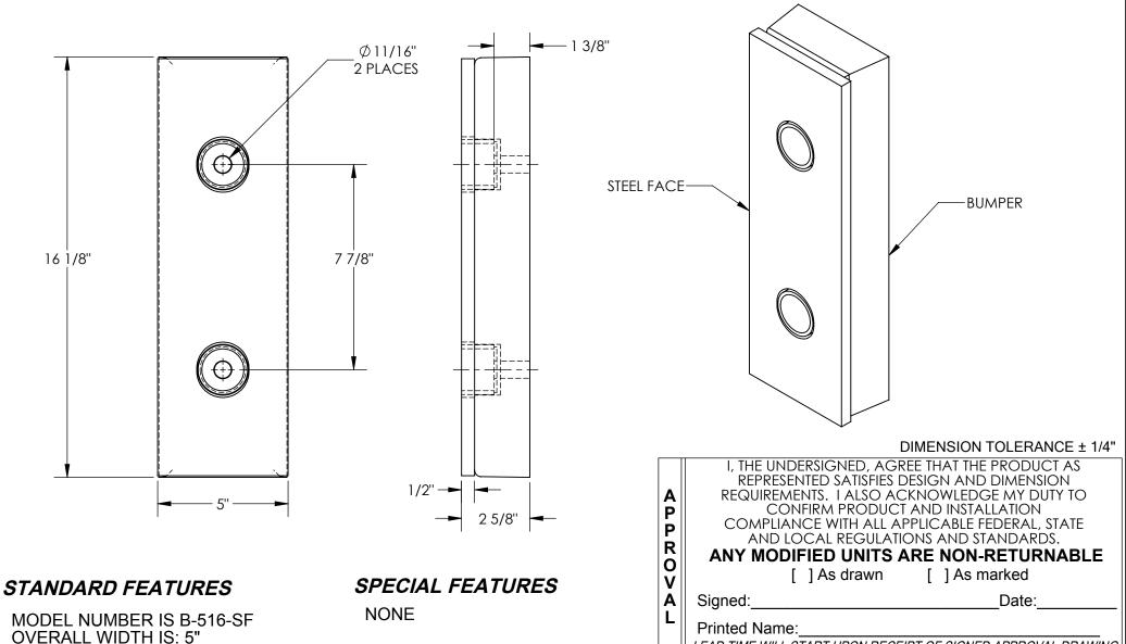
**OVERALL DEPTH IS: 25/8"** STEEL FACE DEPTH IS: 1/2" **OVERALL HEIGHT IS: 16 1/8"** (2) Ø5/8" MOUNTING HOLES \*\*MOUNTING HARDWARE IS NOT INCLUDED\*\*
