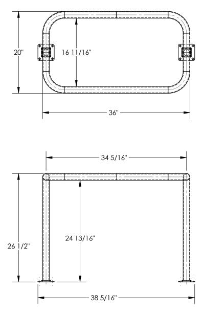
STANDARD FEATURES MODEL NUMBER IS BR-ST-BK **OVERALL WIDTH IS 20" OVERALL LENGTH IS 38 5/16" OVERALL HEIGHT IS 26 1/2"** SPECIAL FEATURES **NONE**
