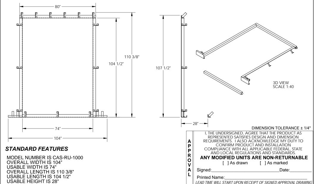
NOTE: UNIT SHIPS UNASSEMBLED. ASSEMBLY TO BE COMPLETED BY THE INSTALLER
