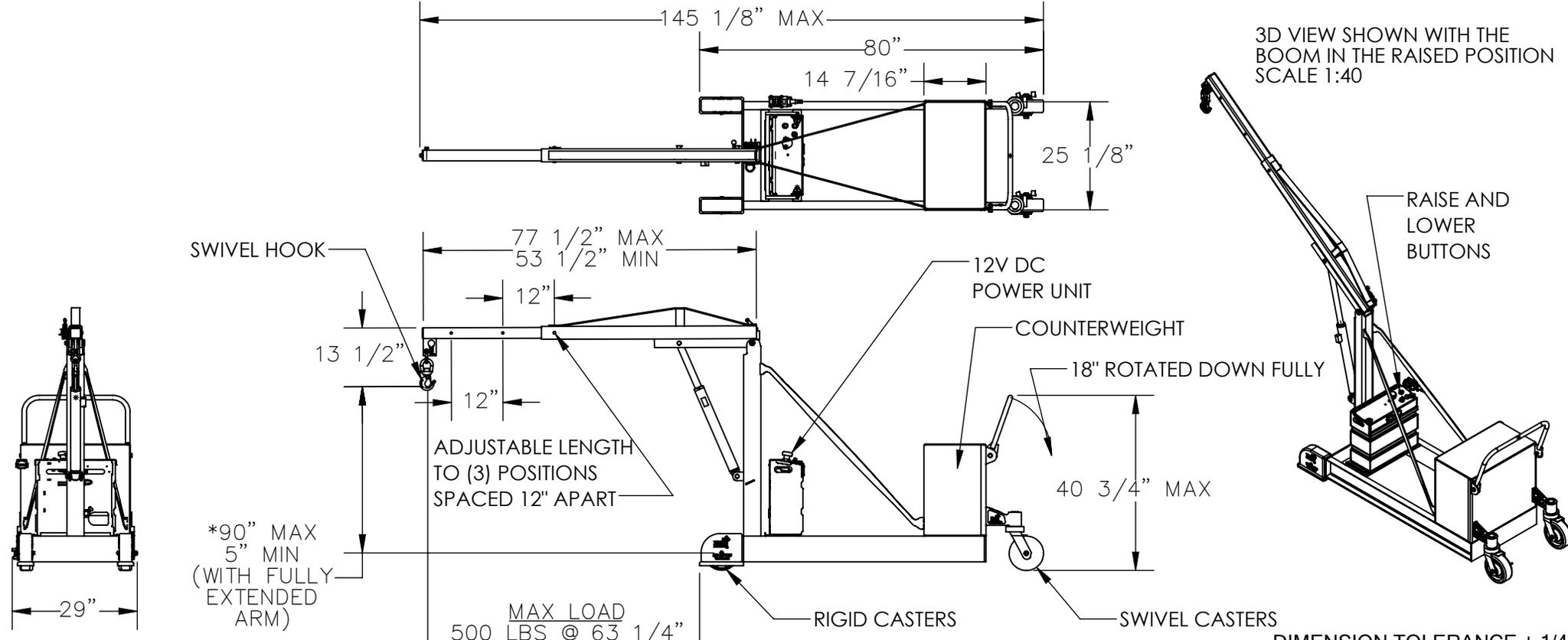
\*WHEN BOOM IS FULLY RETRACTED AND THE CYLINDER IS FULLY RETRACTED HOOK HEIGHT IS 16 7/16"
