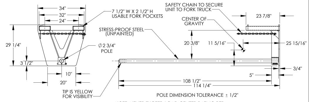
HORIZONTAL CENTER OF GRAVITY: 25 15/16" VERTICAL CENTER OF GRAVITY: 11 5/16" LOST LOAD: 458 LBS. (APPROX.)
