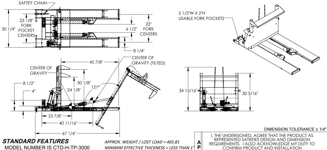
MODEL NUMBER IS CTD-H-TP-3000 OVERALL WIDTH IS 30 1/4" OVERALL LENGTH IS 67 1/4" **USABLE LENGTH IS 45 7/8" OVERALL HEIGHT IS 34 15/16" USEBLE HEIGHT IS 24 1/8" OVERALL TILT IS 121°** MAX CAPACITY IS 3000 LBS USABLE FORK POCKETS: 5 1/2"W X 2"H DURABLE LIQUID PAINT YELLOW FINISH MINIMUM 2400 PSI, MAXIMUM 3000 PSI FOR 3000 LBS CAPACITY FORK LIFT AUXILIARY CONNECTIONS ARE REQUIRED FOR USE
