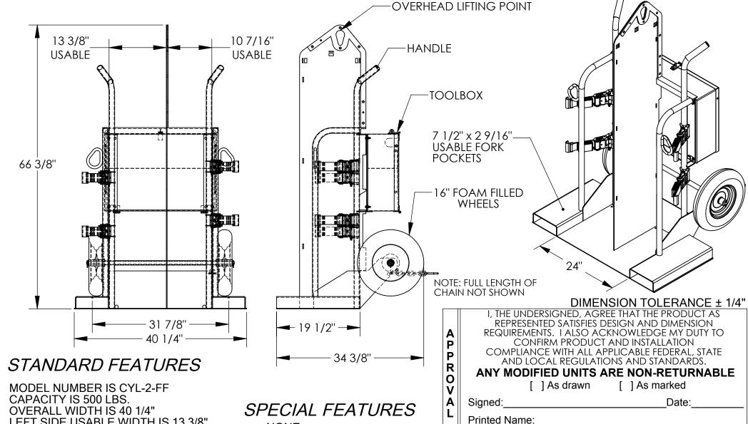
LEFT SIDE USABLE WIDTH IS 13 3/8" RIGHT SIDE USABLE WIDTH IS 10 7/16" **OVERALL DEPTH IS 34 3/8" OVERALL HEIGHT IS 66 3/8"** 7 1/2"W x 2 9/16"H USABLE FORK POCKETS STRAPS TO SECURE TANKS SAFETY CHAIN TO SECURE UNIT TO FORK TRUCK 16" FOAM FILLED WHEELS
