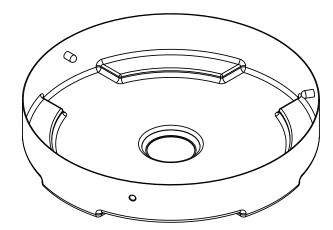
STANDARD FEATURES MODEL NUMBER IS DC-P-55-CAN-BK OVERALL DIAMETER IS  $\emptyset$  24 3/4" **OVERALL HEIGHT IS** 5 1/4" DIAMETER OF OPENING IS  $\emptyset 4$ " MADE FROM LOW-DENSITY POLYETHYLENE DETENTS HOLD LID SECURELY IN PLACE COLOR IS BLACK WORKS WITH 55 GALLON, CLOSED HEAD DRUMS.
