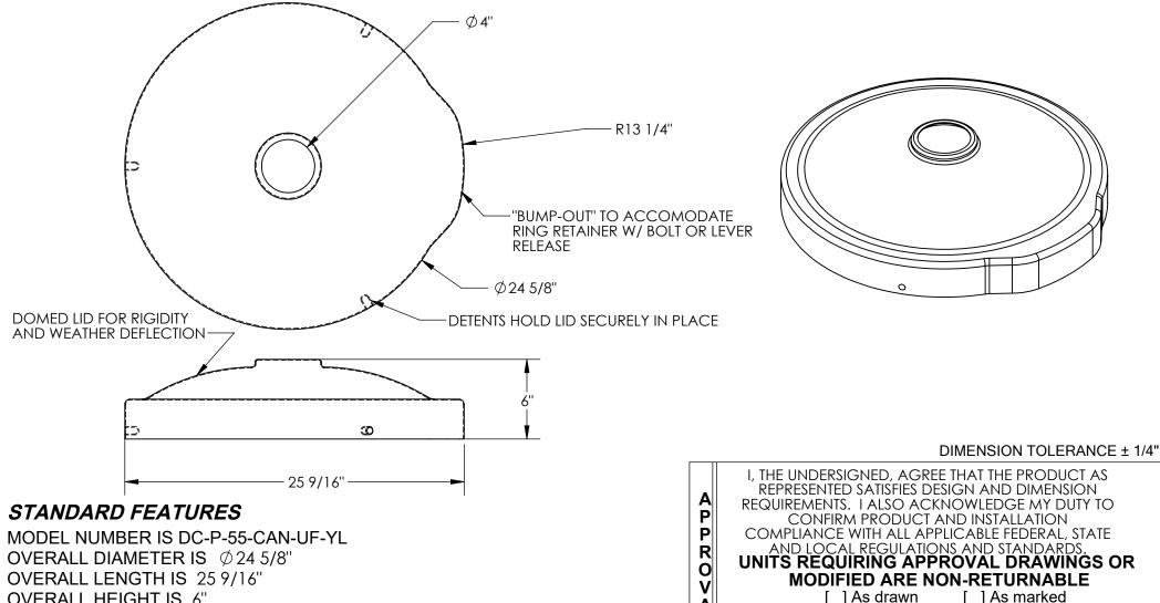
OVERALL HEIGHT IS 6" MADE FROM LOW-DENSITY POLYETHYLENE DETENTS HOLD LID SECURELY IN PLACE DOMED LID FOR RIGIDITY AND WEATHER DEFLECTION "BUMP-OUT" ON OUTER DIAMETER WILL ACCOMODATE RING RETAINER.
