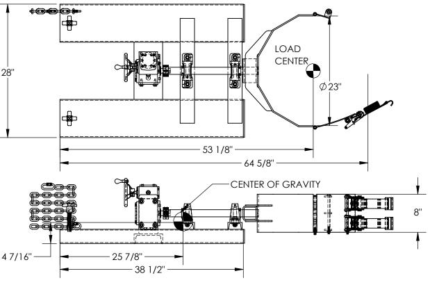
APPROX. WEIGHT / LOST LOAD = 259 LBS. MINIMUM EFFECTIVE THICKNESS = FORK LENGTH MINUS 38 1/2" NEVER EXCEED LOAD CENTER RATING PER FORKTRUCK MANUFACTURERS GUIDELINES. DO NOT USE THIS FORK TRUCK ATTACHMENT IF LOAD WILL EXCEED FORK TRUCK MANUFACTURER'S LOAD CENTER RATING
