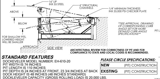
ALL STRUCTURAL STEEL CONSTRUCTION WELDING MEETS AWS.
