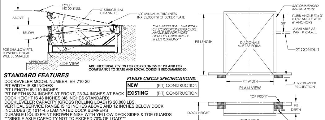
ALL STRUCTURAL STEEL CONSTRUCTION WELDING MEETS AWS.
