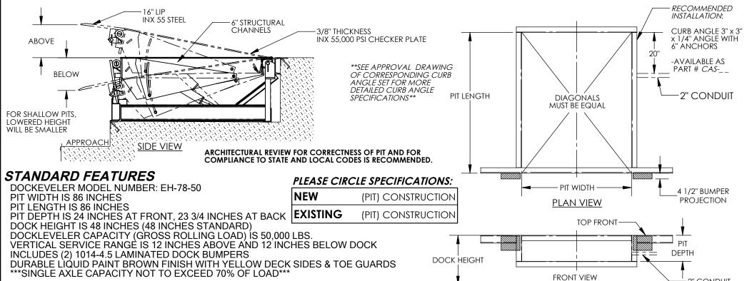
ALL STRUCTURAL STEEL CONSTRUCTION WELDING MEETS AWS.
