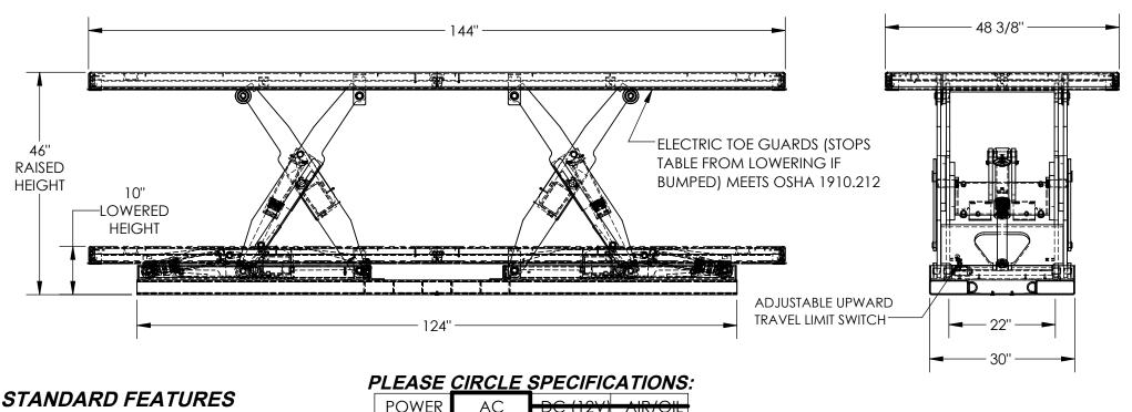
MODEL NUMBER IS EHLT-TL-48144-2-46 PLATFORM WIDTH: 48 3/8" PLATFORM LENGTH: 144" PLATFORM RAISED HEIGHT: 46" PLATFORM LOWERED HEIGHT: 10" TABLE CAPACITY (EVENLY DISTRIBUTED) LOAD: 2.000 LBS.
