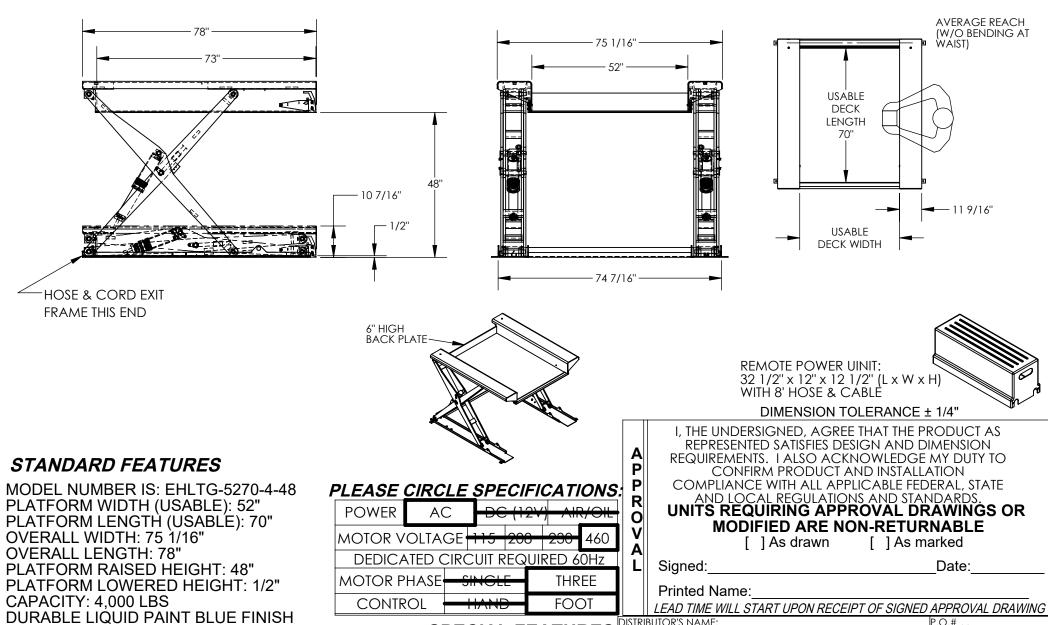
CONTROL IS FOOT SWITCH, 2 PEDAL, NEMA 1
