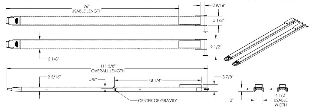
STANDARD FEATURES **MODEL NUMBER IS FE-4-108-P-RS OVERALL WIDTH IS 5 1/8" OVERALL WIDTH W/PIN IS 9 1/2" USABLE WIDTH IS 4 1/2" OVERALL LENGTH IS 111 5/8" USABLE LENGTH IS 96" OVERALL HEIGHT IS 3 7/8"** FITS 4" WIDE x 2" MAX. THICKNESS FORK SOLID STEEL CONSTRUCTION TOUGH BAKED IN POWDER COATED YELLOW FINISH
