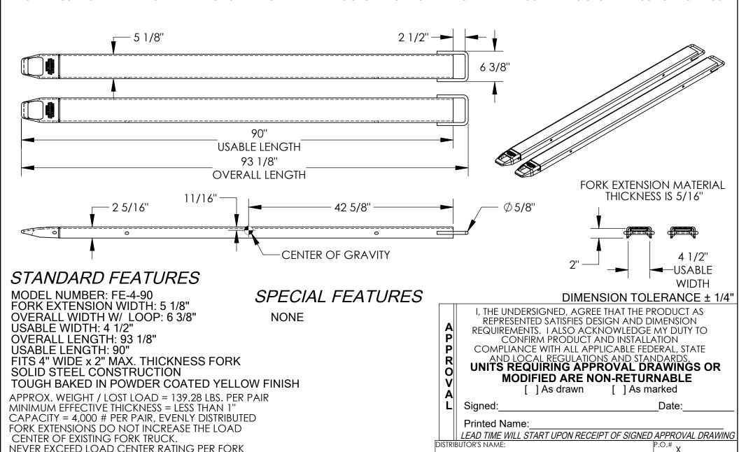
TRUCK MANUFACTURER'S GUIDELINES. VESTIL MANUFACTURING DO NOT USE THESE FORK EXTENSIONS IF LOAD WILL DRAWN BY: S.ROSE EXCEED FORK TRUCK MANUFACTURER'S LOAD CENTER RATING. REFERENCE: FORK EXTENSIONS MUST NOT EXCEED 150% ORIGINAL FORK LENGTH. Quoted lead time:  $_{f Y}$
