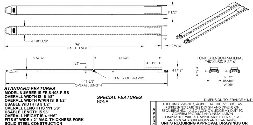
TOUGH BAKED IN POWDER COATED YELLOW FINISH APPROX. WEIGHT / LOST LOAD = 203.73 LBS. PER PAIR MINIMUM EFFECTIVE THICKNESS = LESS THAN 1" CAPACITY = 4,000 # PER PAIR, EVENLY DISTRIBUTED FORK EXTENSIONS DO NOT INCREASE THE LOAD CENTER OF EXISTING FORK TRUCK. NEVER EXCEED LOAD CENTER RATING PER FORK TRUCK MANUFACTURER'S GUIDELINES. DO NOT USE THESE FORK EXTENSIONS IF LOAD WILL EXCEED FORK TRUCK MANUFACTURER'S LOAD CENTER RATING. FORK EXTENSIONS MUST NOT EXCEED 150% ORIGINAL FORK LENGTH.
