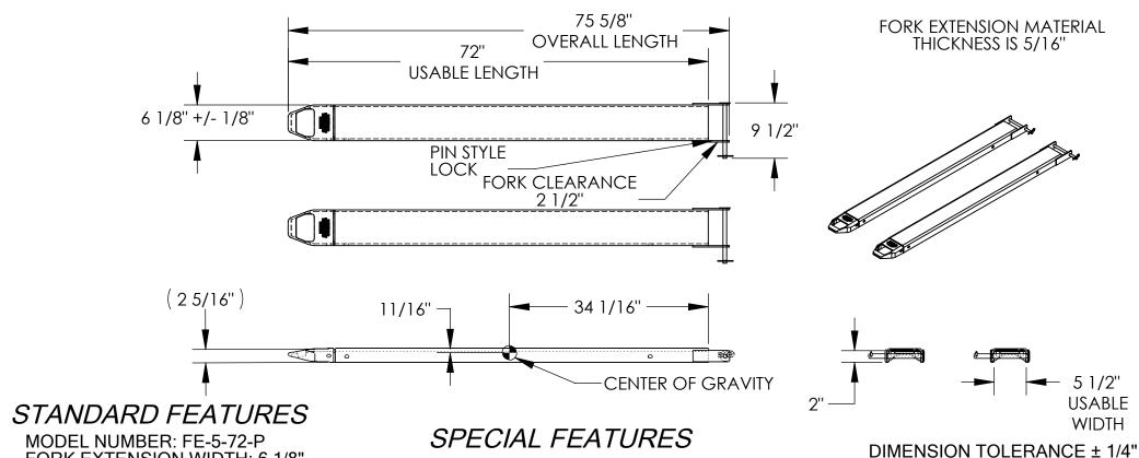
FORK EXTENSION WIDTH: 6 1/8" OVERALL WIDTH W/ RETAINING PIN: 9 1/2"
