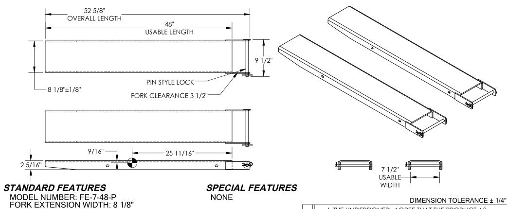
**OVERALL WIDTH W/ RETAINING PIN: 9 1/2"**
