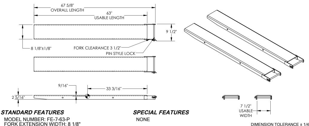
OVERALL WIDTH W/ RETAINING PIN: 9 1/2" **USABLE WIDTH: 7 1/2"**
