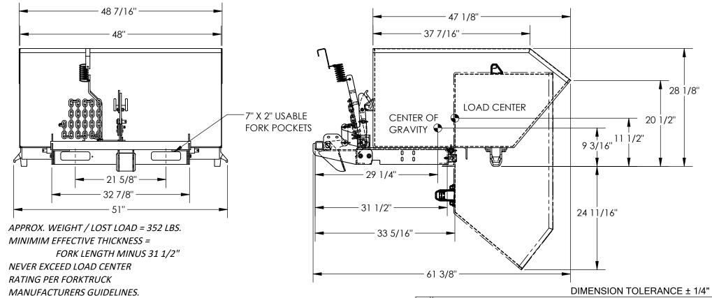
\*\* ADDITION OF CASTERS MAY DO NOT USE THIS FORK TRUCK CHANGE WEIGHT CAPACITY ATTACHMENT IF LOAD WILL **BASED ON CASTER RATING** EXCEED FORK TRUCK MANUFACTURER'S
