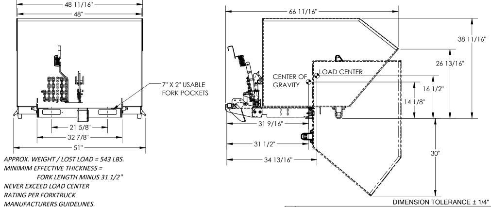
ATTACHMENT IF LOAD WILL EXCEED FORK TRUCK MANUFACTURER'S LOAD CENTER RATING
