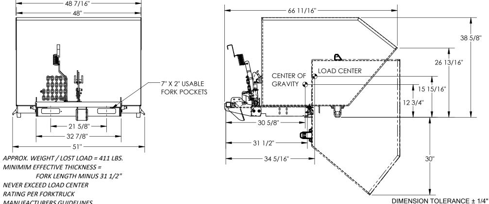
MANUFACTURERS GUIDELINES. DO NOT USE THIS FORK TRUCK ATTACHMENT IF LOAD WILL EXCEED FORK TRUCK MANUFACTURER'S LOAD CENTER RATING
