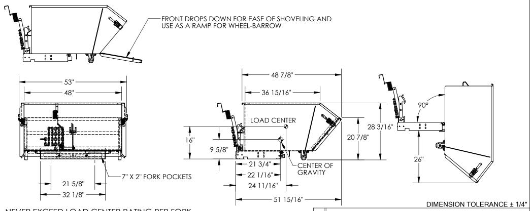
NEVER EXCEED LOAD CENTER RATING PER FORK TRUCK MANUFACTURER'S GUIDELINES. DO NOT USE THIS FORK TRUCK ATTACHMENT IF LOAD WILL EXCEED FORK TRUCK MANUFACTURER'S LOAD CENTER RATING. APPROX. WEIGHT/LOST LOAD=411.95 LBS. EFFECTIVE THICKNESS= FORK LENGTH MINUS 21 3/4"
