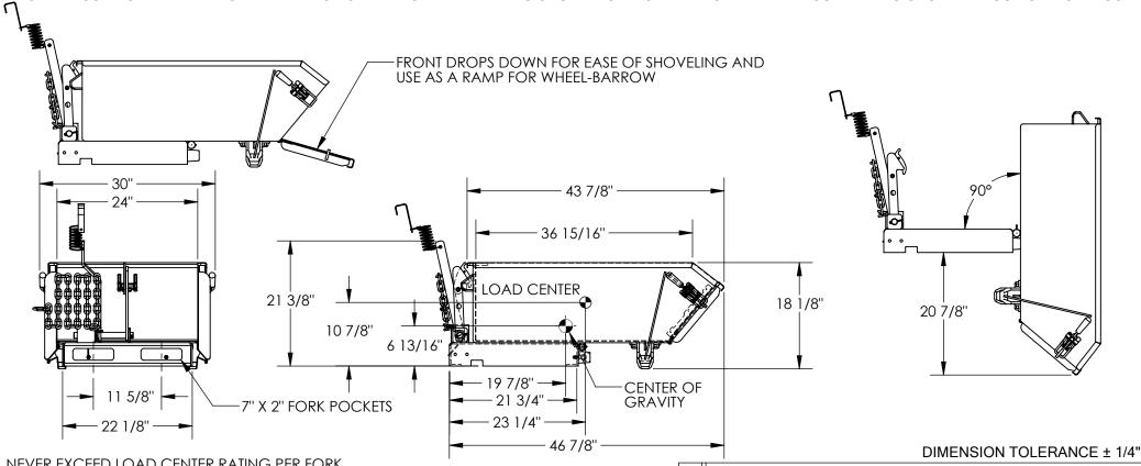
NEVER EXCEED LOAD CENTER RATING PER FORK TRUCK MANUFACTURER'S GUIDELINES. DO NOT USE THIS FORK TRUCK ATTACHMENT IF LOAD WILL EXCEED FORK TRUCK MANUFACTURER'S LOAD CENTER RATING. APPROX. WEIGHT/ LOST LOAD=200.34 LBS.
