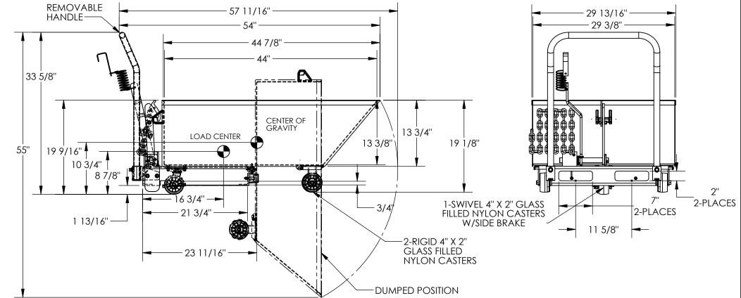
NEVER EXCEED LOAD CENTER RATING PER FORK TRUCK MANUFACTURER'S GUIDELINES. DO NOT USE THIS FORK TRUCK ATTACHMENT IF LOAD WILL EXCEED FORK TRUCK MANUFACTURER'S LOAD CENTER RATING. APPROX. WEIGHT/ LOST LOAD=209.10 LBS.
