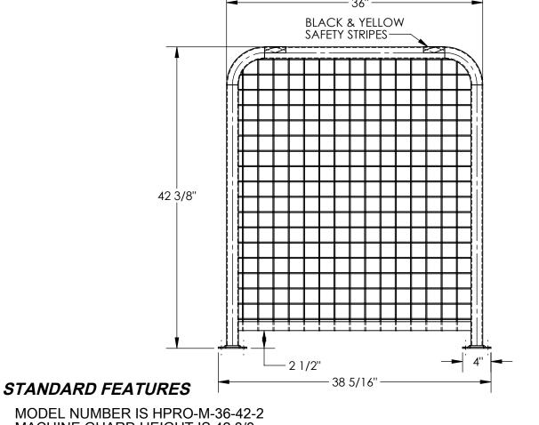
MODEL NUMBER IS HPRO-M-36-42-2 MACHINE GUARD HEIGHT IS 42 3/8 MACHINE GUARD LENGTH IS 36" MACHINE GUARD DIAMETER IS: Ø1 11/16" MESH HEIGHT FROM GROUND: 2 1/2" OVERALL LENGTH: 38 5/16" **INCLUDES 2 MOUNTING BRACKETS** TOUGH BAKED IN POWDER COATED YELLOW FINISH BLACK AND YELLOW SAFETY STRIPES ALL STEEL CONSTRUCTION (ASTM A-36 MIN.) WITH WELDING TO MEET AWS WARNING: CHECK APPLICABLE STATE & LOCAL LAWS FOR YOUR AREA
