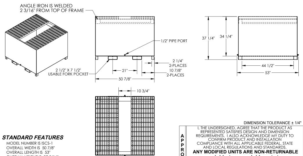
OVERALL HEIGHT IS 37 5/16" FORK POCKET CENTER TO CENTER IS 21" USABLE FORK POCKET SIZE IS 2 1/2" X 7 1/2" GRATE SPACING IS 10 3/4" MAX WEIGHT CAPACITY IS 2,500 LBS MAX FLUID CAPACITY IS 400 GALLONS WEIGHT WHEN FULL CAPACITY IS 4,362 LBS WEIGHT WHEN EMPTY IS 1,018 LBS **GRATING IS REMOVABLE** DURABLE LIQUID PAINT YELLOW FINISH
