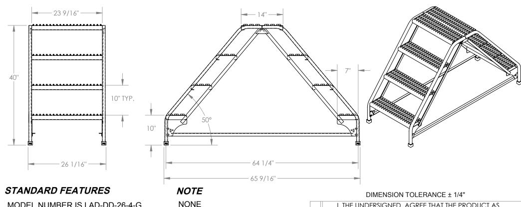
MODEL NUMBER IS LAD-DD-26-4-G OVERALL WIDTH IS 26 1/16" USABLE WIDTH IS 23 9/16" **OVERALL LENGTH IS 65 9/16" USABLE LENGTH IS 64 1/4" OVERALL HEIGHT IS 40"** STEP DEPTH IS 7" **TOP PLATFORM DEPTH IS 14"** ANGLE OF INCLINE IS 50° STEP STYLE IS GRIP STRUT **COLOR IS VESTIL BLUE** MAX CAPACITY IS 350 LBS
