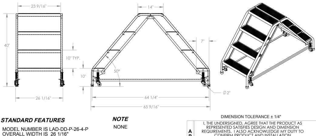
OVERALL WIDTH IS 26 1/16" USABLE WIDTH IS 23 9/16" OVERALL LENGTH IS 65 9/16" USABLE LENGTH IS 64 1/4" OVERALL HEIGHT IS 40" STEP DEPTH IS 7" TOP PLATFORM DEPTH IS 14" ANGLE OF INCLINE IS 50° STEP STYLE IS PERFORATED COLOR IS VESTIL YELLOW MAX CAPACITY IS 350 LBS WHEEL SIZE IS Ø 2"
