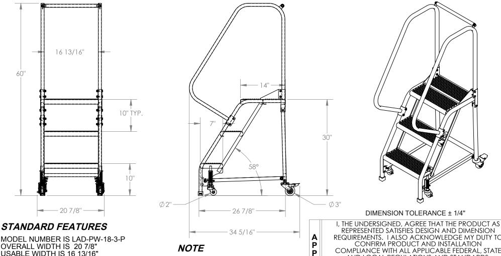
MODEL NUMBER IS LAD-PW-18-3-P OVERALL WIDTH IS 20 7/8" **USABLE WIDTH IS 16 13/16"** OVERALL LENGTH IS 34 5/16" **USABLE LENGTH IS 26 7/8" OVERALL HEIGHT IS 60"** PLATFORM HEIGHT IS 30" **COLOR IS VESTIL BLUE** STEP TYPE IS PERFORATED CLIMB ANGLE IS 58° STEP DEPTH IS 7" PLATFORM DEPTH IS 14" MAX CAPACITY IS 350 LBS FRONT Ø2" DIRECTIONAL SPRING-LOADED SWIVEL CASTERS
