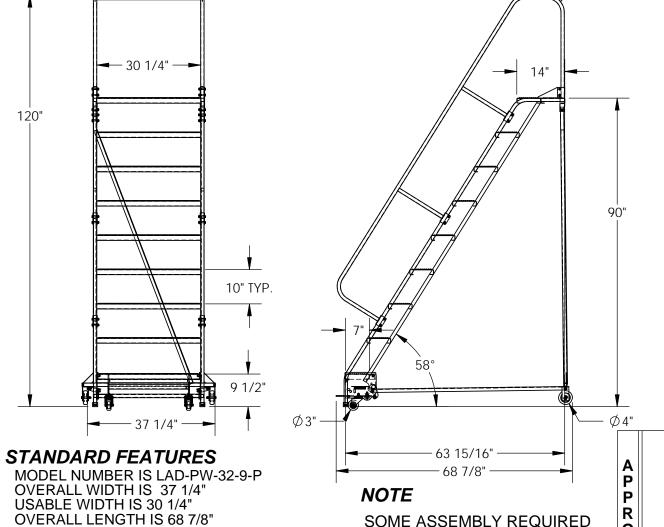
USABLE LENGTH IS 63 15/16" **OVERALL HEIGHT IS 120"** PLATFORM HEIGHT IS 90" STEP TYPE IS PERFORATED CLIMB ANGLE IS 58° STEP DEPTH IS 7" PLATFORM DEPTH IS 14" **COLOR IS VESTIL BLUE BOTTOM STEP COLOR IS YELLOW** MAX CAPACITY IS 350 LBS FRONT WHEEL IS SWIVEL, SIZE IS Ø 3" REAR WHEEL IS RIGID, SIZE IS Ø 4"
