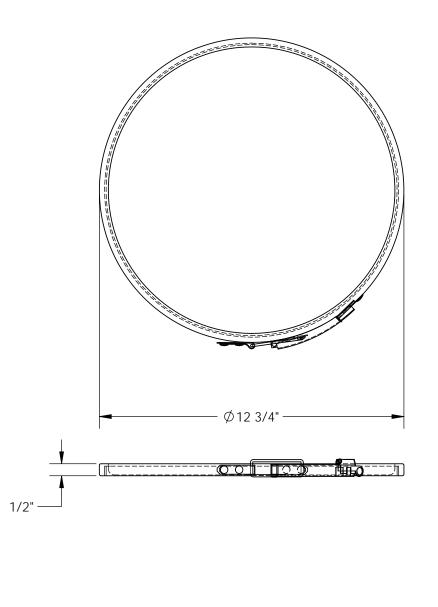
STANDARD FEATURES MODEL NUMBER IS LID-STL-LL OVERALL WIDTH IS 1/2" LID DIAMETER IS Ø12 3/4" SPECIAL FEATURES NONE
