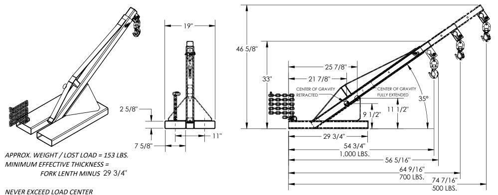
RATING PER FORKTRUCK MANUFACTURERS GUIDELINES. DO NOT USE THIS FORK TRUCK ATTACHMENT IF LOAD WILL EXCEED FORK TRUCK MANUFACTURER'S LOAD CENTER RATING
