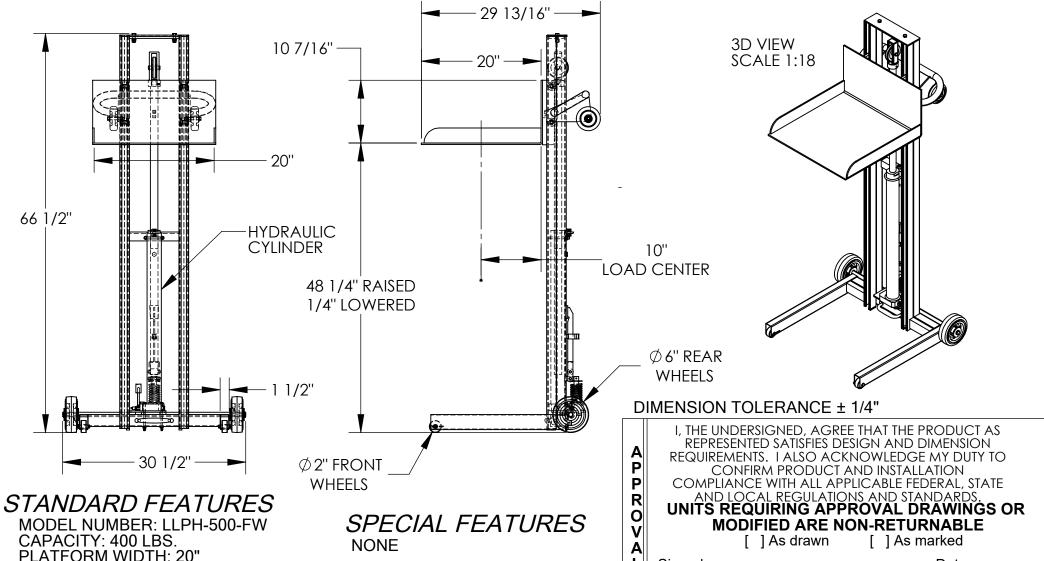
PLATFORM WIDTH: 20" PLATFORM LENGTH: 20" OVERALL WIDTH: 30 1/2" OVERALL LENGTH: 29 13/16"
