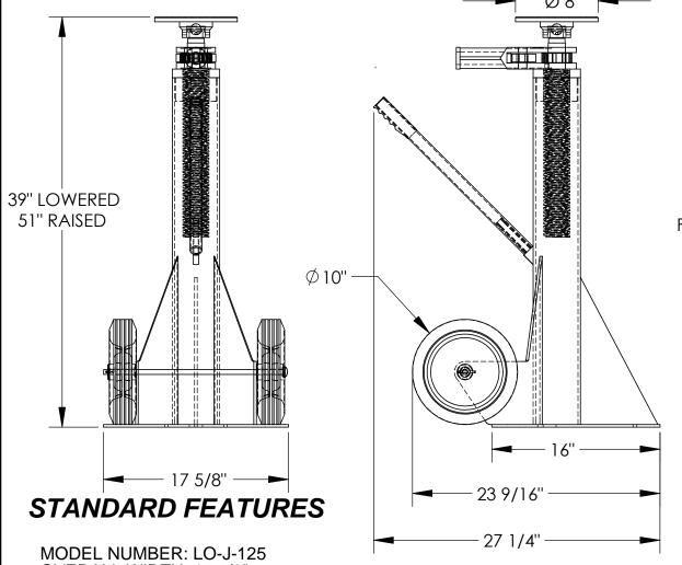
MODEL NUMBER: LO-J-125 OVERALL WIDTH: 17 5/8" OVERALL LENGTH: 27 1/4" SERVICE RANGE: 39" TO 51" STATIC CAPACITY: 125,000 LBS. LIFTING CAPACITY: 50,000 LBS.
