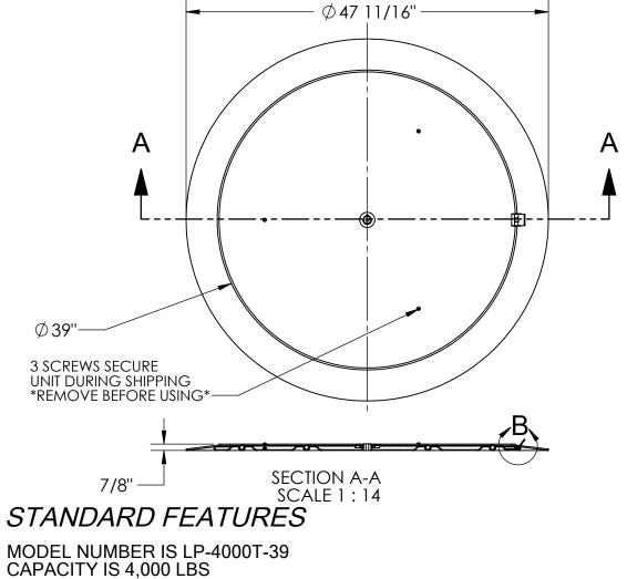
MODEL NUMBER IS LP-4000T-39 CAPACITY IS 4,000 LBS USEABLE DIAMETER IS 39" OVERALL DIAMETER IS 47 11/16" OVERALL HEIGHT IS 7/8" STARTING FORCE: 35 LBS @ 4,000 LBS MAINTAIN FORCE: 25 LBS @ 4,000 LBS DURABLE LIQUID PAINT BLUE FINISH
