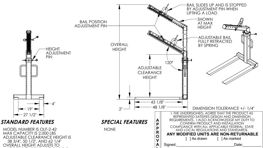
62 9/16", 74 5/16", AND 86 1/16" FORKS ARE FIXED/ NON ADJUSTABLE FORK SIZE IS 2" H X 4" W **USABLE FORK LENGTH IS 43 1/8" OVERALL WIDTH IS 27 1/2"** OVERALL LENGTH IS 48 1/8" **DURABLE LIQUID PAINT BLUE FINISH**
