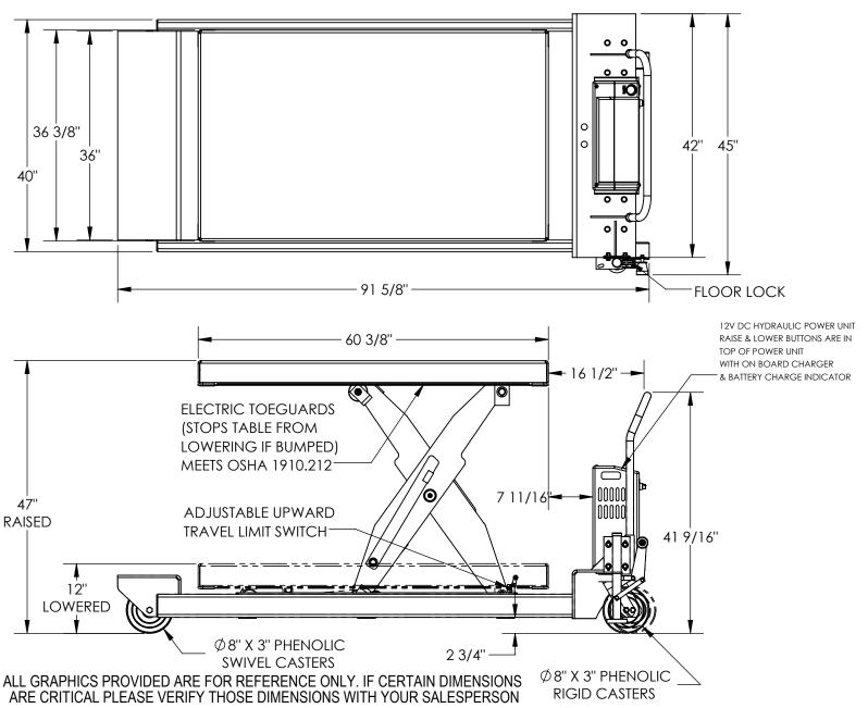
DIMENSION TOLERANCE ± 1/2" TABLE HEIGHT TOLERANCE ± 1/2" DECK FLATNESS ± 1/4'
