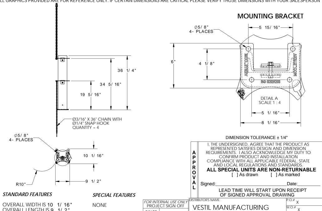
OVERALL LENGTH IS 9 1/2" OVERALL HEIGHT IS 36 1/4" COMPATIBLE CYLINDERS: Ø9" TO Ø12" TWO CYLINDERS CAN BE STORED
