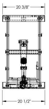
DECK TOLERANCE ±1/2" TABLE HEIGHT TOLERANCES ±1/2" DECK FLATNESS ±1/4"
