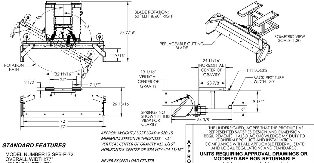
**OVERALL WIDTH:77" USABLE WIDTH: 72" OVERALL LENGTH: 54 3/8" OVERALL HEIGHT:26 13/16"** FORK POCKETS: 2 1/2" X 7 1/2" **SNOW BLADE WIDTH: 72"**
