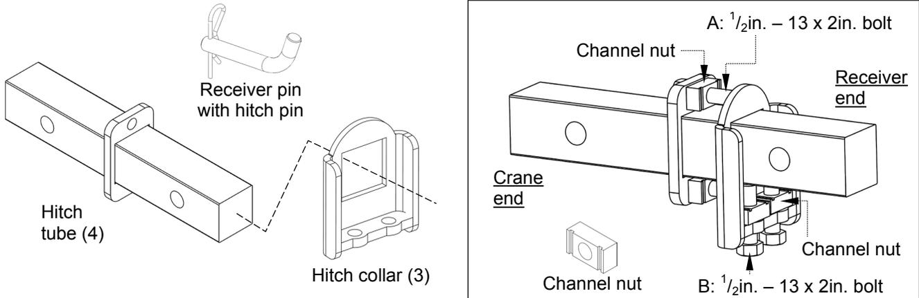
**Step 1B:** Insert the receiver end of the hitch tube into the receiver of your trailer hitch. Pin the hitch bar to the receiver using the receiver pin and pin clip (items 16 & 30). Next, slide the collar around the end of the receiver and tighten the bolts (B) firmly against the bottom of the receiver.
