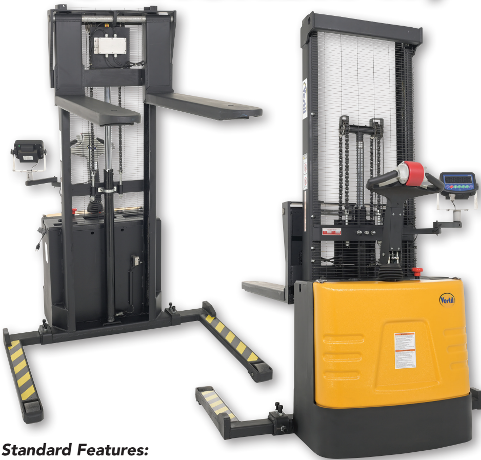
DIGITAL SCALE READOUT PROVIDES WEIGHT IN POUNDS OR KILOGRAMS
