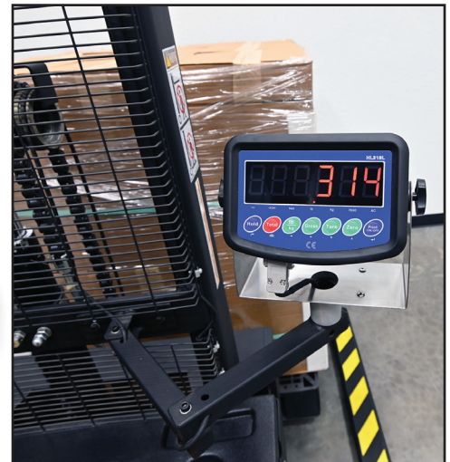
DIGITAL SCALE READOUT PROVIDES WEIGHT IN POUNDS OR KILOGRAMS
