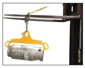
**To Use:** Simply attach the lifter to a lifting device, such as a fork truck, by utilizing the centrally located chain/hook opening. Once the unit is secured, place the arms tightly under the top and base ridges of the LP tank, lift to desired height, and transport to the preferred location.
