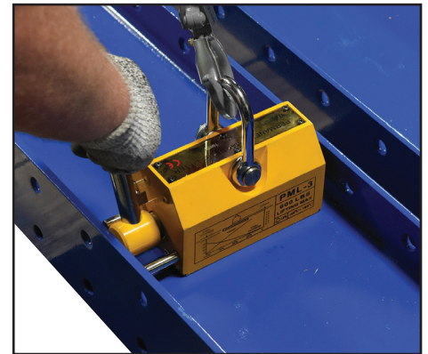
Magnets Activated/Deactivated by Simple Lever Rotation
