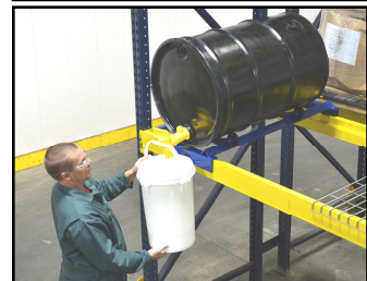
Drum rests on rollers & can be rotated to dispensing position
